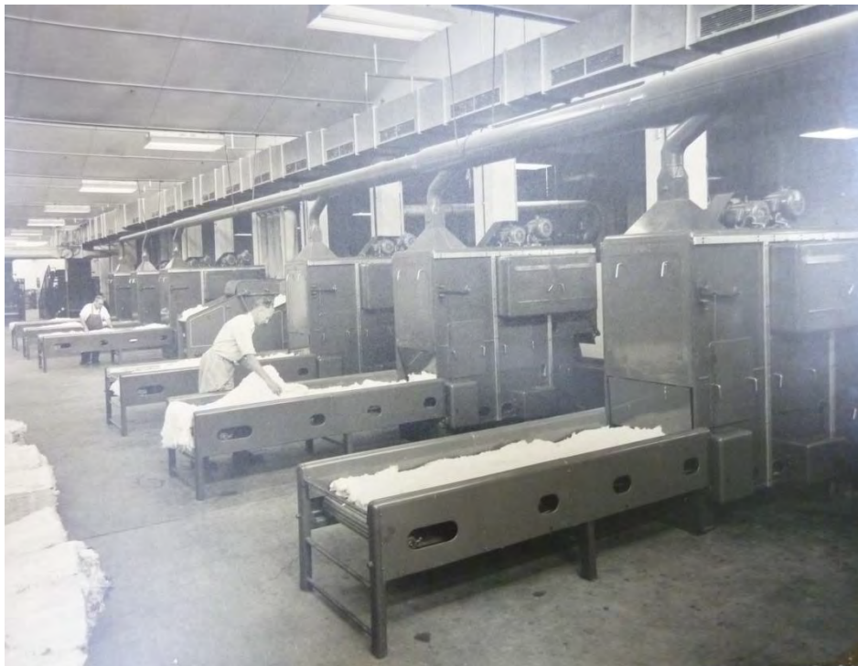
Figure 38 The cotton 'fleeces' after they have been through the first stage of processing. (Source: Pacific Brands archives)
