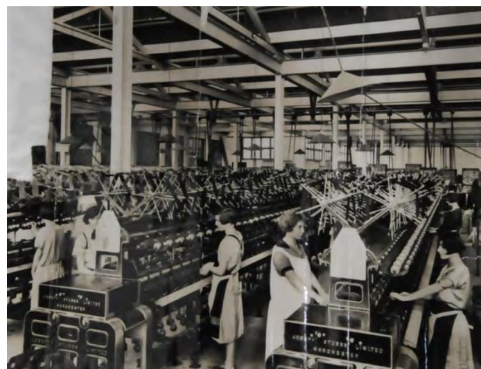
Figure 8 Winding from skein to bobbin, Bonds Wentworthville 1927. (Source: Pacific Brands archives)
